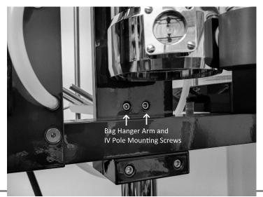
PRO TIP: Before tightening the Bag Hanger Arm completely, install the IV Pole and extend as tall as possible. Using the IV Pole as a vertical guide, hold the Bag Hanger arm straight, keep the IV Pole as vertical as possible, and tighten the Bag Arm Mounting Screws. Take a step back and admire your handiwork. If the IV Pole is leaning to the left or right, loosen one of the two Mounting screws, rotate the Bag Hanger Arm until the IV Pole is no longer leaning, and retighten the Mounting Screws.
