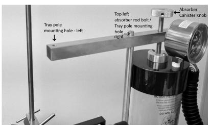
Loosen the **Absorber Canister Knob** and remove the soda sorb canister for this procedure. Using the enclosed 3/16<sup>th</sup> Allen wrench remove the **Top Left Absorber Rod Bolt. This bolt can be discarded.** This will reveal the **Tray Pole Mounting Hole-right.**
