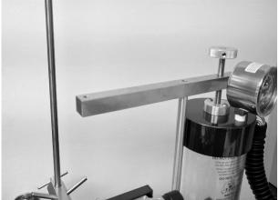
Place both Tray mounting poles into the mounting holes (right and left) and tighten completely (best if done by hand to avoid scratching the brushed aluminum surface). There should now be two mounting poles (Left and Right), one top **right** absorber rod bolt (never removed) in place.
