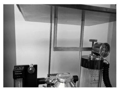
The **Bag Hanger Arm and IV Pole Combo** is mounted on the back of the vaporizer mounting plate. The **Mounting Screws** are installed from the front of the vaporizer plate, through the plate and into the **Bag Hanger Arm**.
