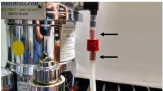
Remove the current opaque silicon hose from the vaporizer outlet adapter which is located on the right (outlet) side of the vaporizer if you are facing the front of the vaporizer.
